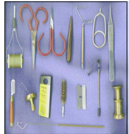
Top left to right ↑ Umpqua Ceramic Bobbin Large Scissors Small Scissors Bodkin Materelli Whip Finish English Hackle Pliers Tweezers Bottom left to right Small Comb Dyna-King Dubbing-Whirl Griffin Hook and Hackle Gauge Bore Cleaner used to pick out dubbing Razor Blade Griffin Rotating Hackle Pliers Elgin Brass Hair Stacker Across the bottom Bird's Dubbing Tool
